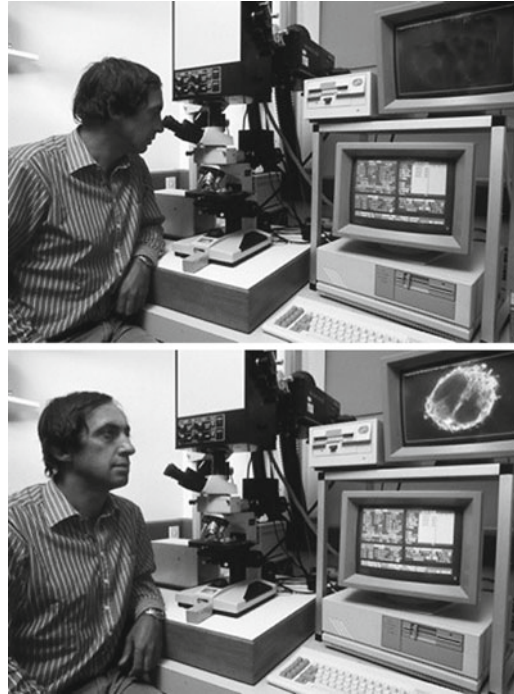
Fig. 2 The author, John White, photographed in the late 1980s seated at an early version of the MRC 500 laser scanning confocal microscope. In the top panel, John is looking into the eyepieces of the fluorescence microscope in order to find a region of interest for scanning. In the lower image the specimen is being scanned by the laser and the image produced by the confocal microscope is visible on the video monitor. The ability to first locate a region of interest by eye using a conventional wide field epifluorescence microscope, and to subsequently scan the same region in the confocal mode, remains a significant practical advantage of the laser scanning confocal microscope
