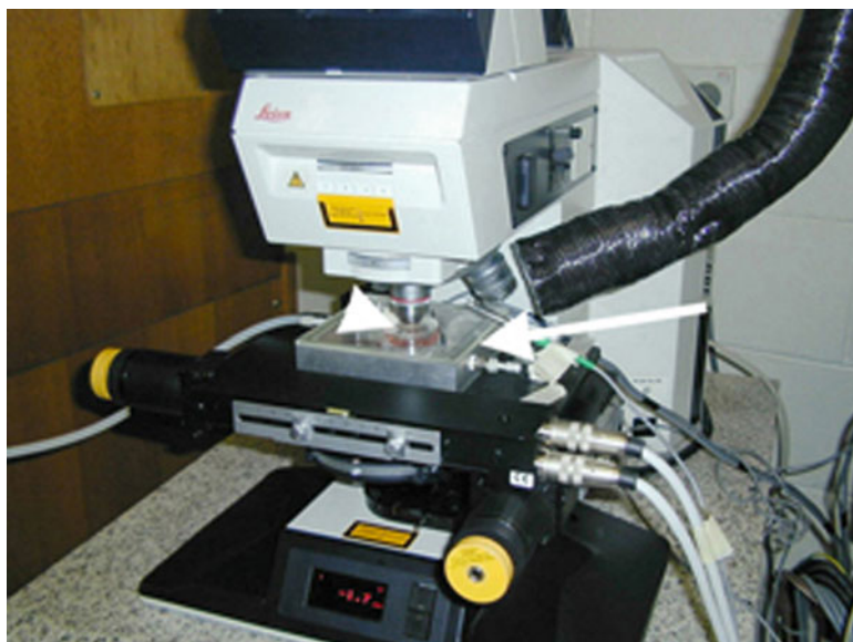
Fig. 6 Environmental chamber on the confocal microscope. Chamber design modified with permission from Frank Costantini. Arrow head indicates Petri dish containing cultured metanephroi. Metanephroi can be cultured for several days in a humidified temperature-controlled chamber ( arrow ) on the confocal microscope
